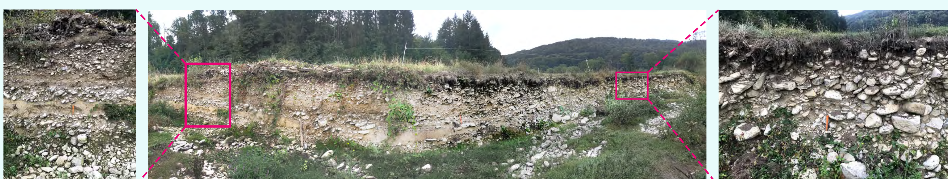
Fig. 7. Outcrop showing intercalation of clayey silt layers with coarse materials.
